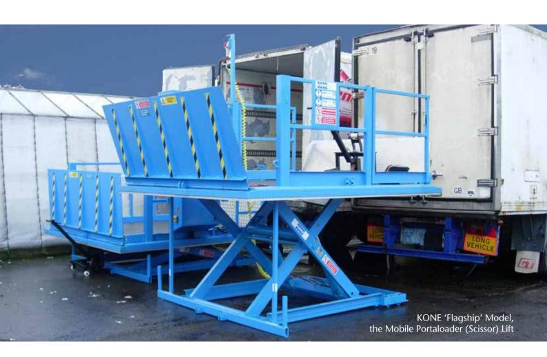
NEW EQUIPMENT, MAINTENANCE, REPAIR SOLUTIONS AND REFURBISHMENT
