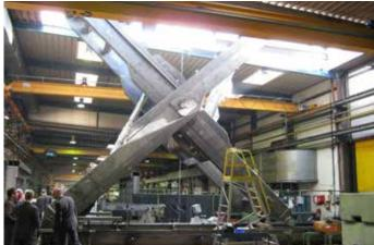
KONE proposed a 30,000 kg capacity scissor lift to perform the 8.9 metres travel from street level down into the building's basement.
