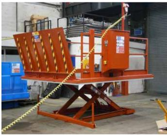
KONE offers two standard scissor lift refurbishment packages, a basic (for a projected additional 10 year lifespan) and a comprehensive (for a projected additional 15 year lifespan and including a 12 month warranty) which we are currently applying at our Keighley factory to a 24 year old UK Lift scissor lift.
