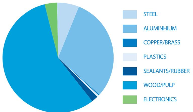
Figure 8. Material structure example for KONE Hermetic Door 30
