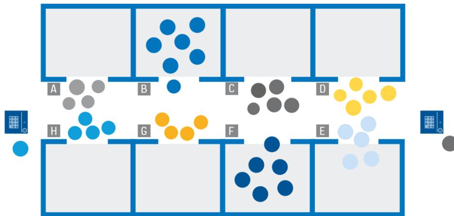
KONE Destination minimises the number of intermediate stops by grouping passengers intelligently. This leads to shorter journey times and better handling capacity compared to conventional full collective lift systems.
