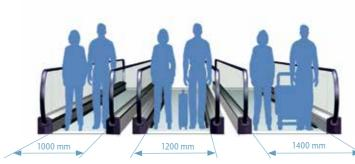
Figure 5.5 Horizontal autowalk pallet widths
