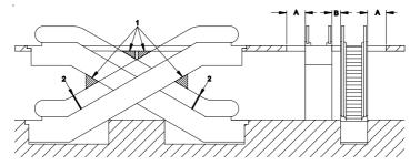
Figure 6.12 Head guards for criss-cross escalators
