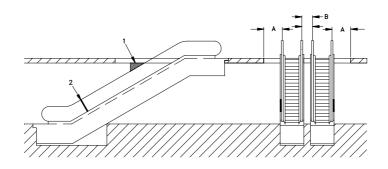
Figure 6.9 Head guards for parallel escalator
