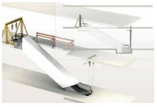
Figure 8.5 Installation using a lifting frame
