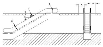
Figure 6.10 Head guards for single escalator
