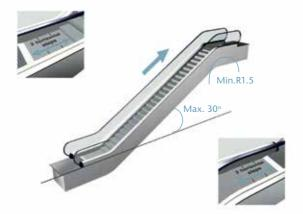
The use of both shopping trolleys and baggage carts on escalators is unsafe and not permitted due to potential misuse, overloading and width restriction. Where shopping trolleys and/or baggage carts are available in the area around escalator installations, suitable barriers should be provided to prevent access with them.
