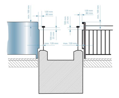
Figure 6.13 Clearances for customer railings according to EN 115-1
