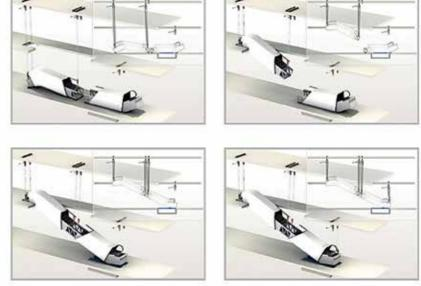
Figure 8.3 Installation in sections is useful when the roof of the building can not be removed
