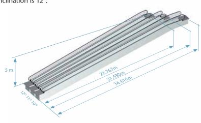
Figure 5.9 The relationship between inclination angle and overall vertical/horizontal dimensions of inclined autowalks.
