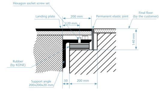
Figure 7.1 Escalator mounting angle
