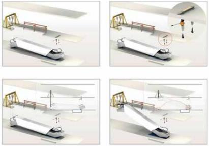
Figure 8.2 Installation in one section using A-frames
