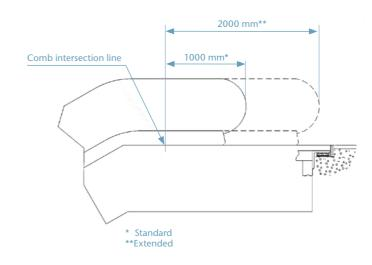
Figure 5.18 Different extended balustrade lengths
