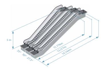
Figure 5.8 The relationship between inclination angle and overall vertical/horizontal dimensions of escalators.
