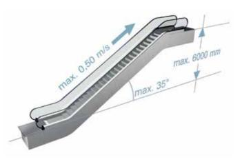
Escalators with a 30° angle of inclination or less are permitted at any step band speed (up to the EN 115-1 maximum of 0.75 m/s) or vertical rise.
