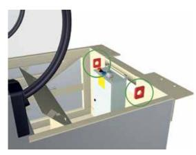
Figure 8.4 Lifting points in the escalator truss
