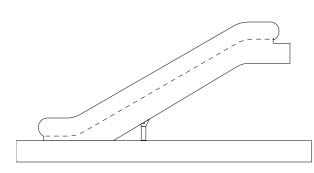
Figure 7.2 Intermediate truss support
