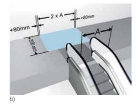
Figure 6.1 a) and b) Passenger circulation area for single escalators A = distance between handrail outer edges
