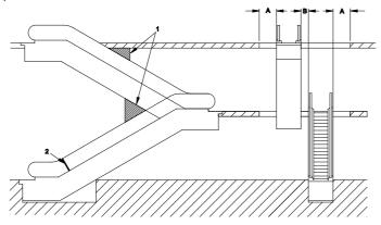
Figure 6.11 Head guards for scissored escalators
