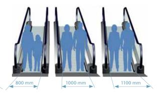
Figure 5.6 Inclined autowalk pallet widths
