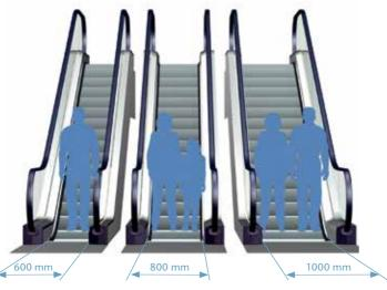
Figure 5.4 Escalator step widths
