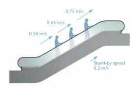
Figure 5.7 The nominal speeds for escalators and autowalks
