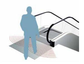
Figure 5.14 Passenger detection by radar or a photocell
