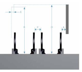
Figure 6.3 Minimum free area around escalators and autowalks
