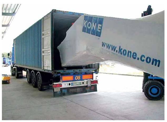
Figure 7.7 Unloading an escalator using forklift trucks
