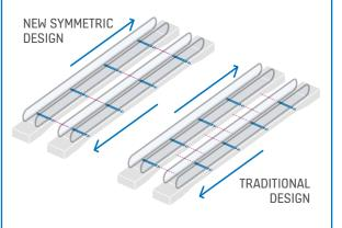
Structural elements and supports are aligned even if parallel autowalks are running in different directions.
